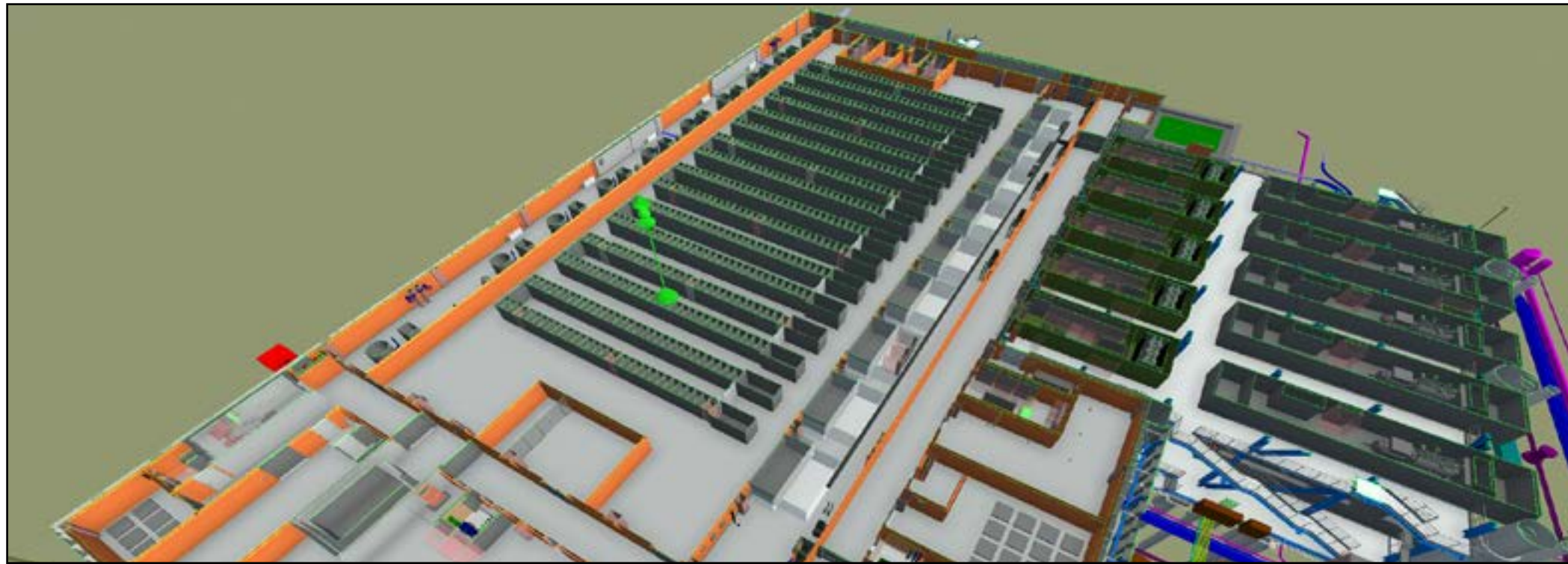
DATA MODULE ROOM, CDU, ELECTRICAL HOUSES, AND GENERATOR UNITS
